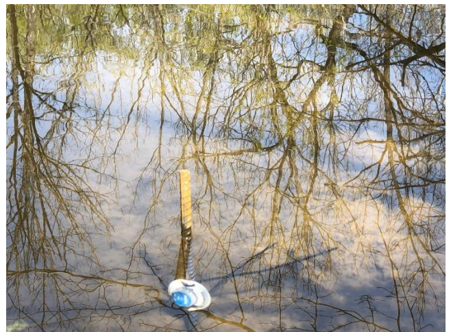
Figure 9: Deployed Data Loggers (DO, Conductivity, pH)
