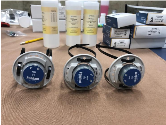
Figure 9: Deployed Data Loggers (DO, Conductivity, pH)
