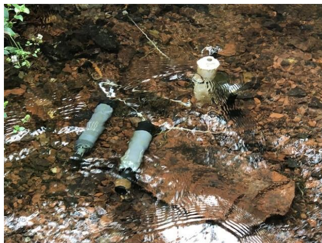
Figure 9: Deployed Data Loggers (DO, Conductivity, pH)
